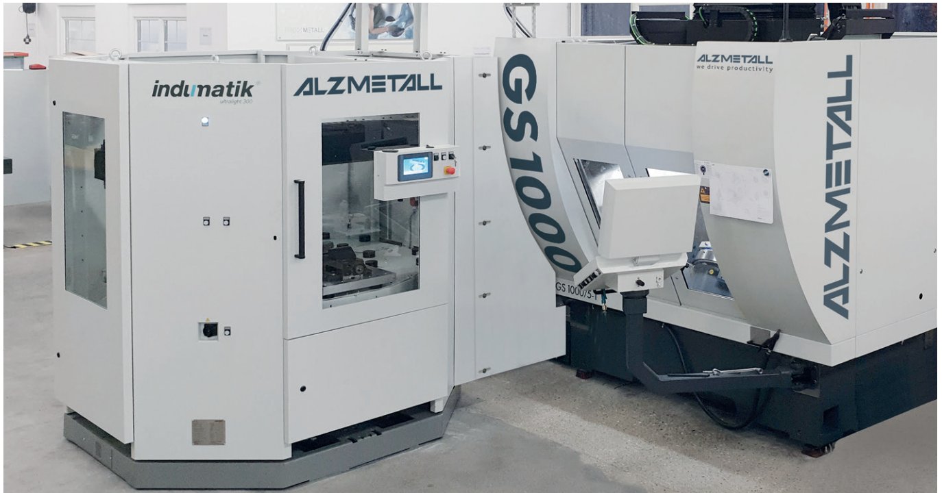
ALZMETALL GS 1000 and INDUMATIK Ultralight 300 implementation. Transfer weight of max. 300 kg, 3-12 pallet positions for pallets 320 x 320 mm up to 630 x 630 mm. Transfer carrier drive for operator access.
